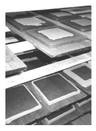
Figure 2.30 Slip coated encaustic tiles left to dry.
