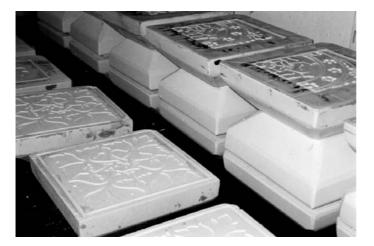
**Figure 2.28** Plaster moulds for encaustic tiles.
