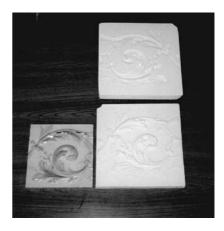
**Figure 2.29** Tiles and mould together showing allowance for shrinkage.
