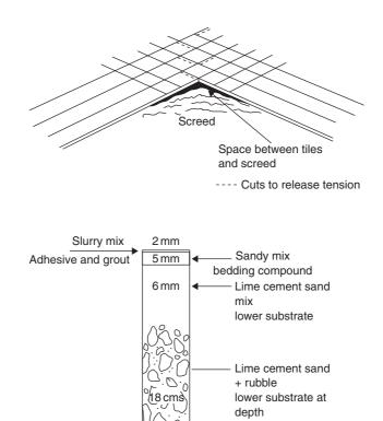
Figure 7.9 Diagram of the cuts used in the tile work under tension.
