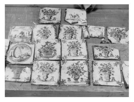
**Figure 5.10** Delft tiles taken from a fireplace showing soot blackening of the edges.
