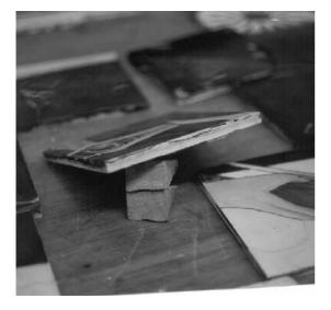
**Figure 5.22** Delamination due to frost action.
