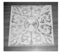
**Figure 2.32** A large slip cast embossed tile with glaze tests applied.
