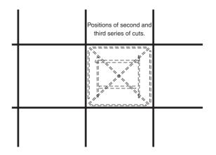
Taking a flat 2 inch cold chisel and a hammer starting at the centre of the tile and working outwards begin to knock away all of the parts of the tile until all that remains is the 3–4 mm of tile which is around the edge. Change to a 1 inch chisel with a thin blade and carefully tap along the grout line holding the chisel at 90 degrees to the tile face. The remaining tile should fall away.
