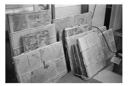
**Figure 7.26** The reverse of the panels after cutting into small sections showing the Portland cement.
