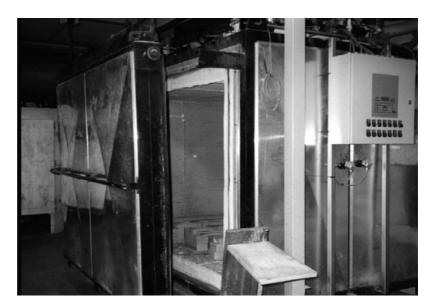
**Figure 2.14** Gas fired kiln for biscuit tiles.
