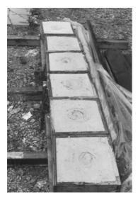
**Figure 5.17** Mortar trials.
