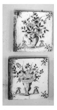
**Figure 2.10** Showing loss of glaze fragments from the edges of the tile, also the extent of soot absorption from use in a fireplace.
