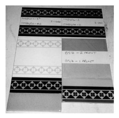
Figure 2.33 Body and glaze colour tests for printed tiles.
