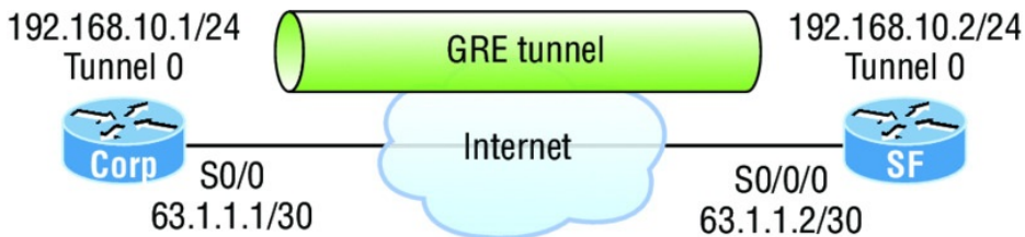
FIGURE 21.24 Example of GRE configuration
