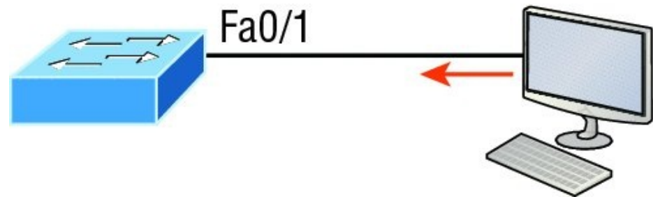
FIGURE 10.6 Protecting a PC in a lobby
