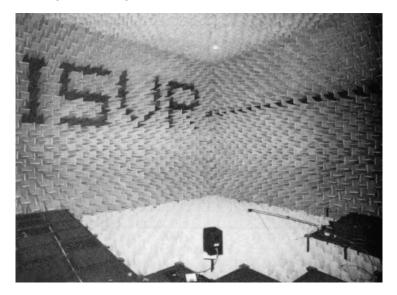
**Figure 2.3** The ISVR anechoic chamber. The large anechoic chamber in the Institute of Sound and Vibration Research at Southampton University, UK, has a volume of  $611 \text{ m}^3$ . The chamber is anechoic down to around 70 Hz. Below this frequency, the wedges represent less than a quarter of a wavelength, and the absorption falls off with decreasing frequency. The floor grids are completely removable, but are strong enough to support the weight of motor vehicles
