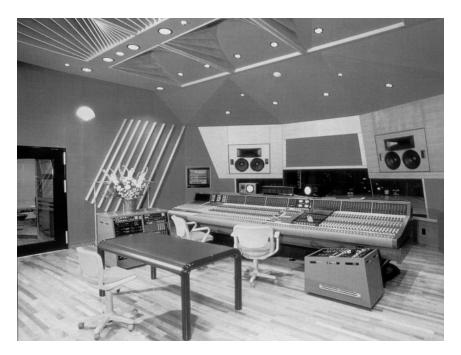
**Figure 18.4** Hitokuchi-Zaka studios, Tokyo, Japan. In this control room, designed by Shozo Kinoshita, all furniture is kept below ear height, and is positioned to avoid confusing reflexions. Although the monitor loudspeakers are mounted relatively high, the size of the room ensures that the monitoring angle is kept low
