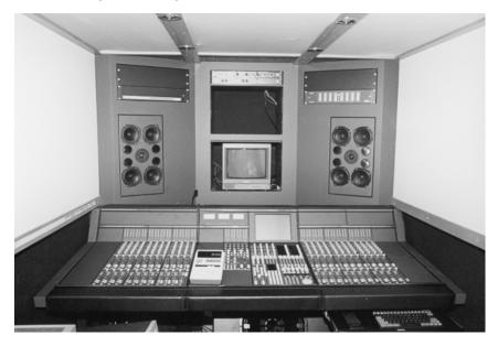
Figure 23.17 The complete front half of the truck, with the sub-woofer just visible below the mixing console
