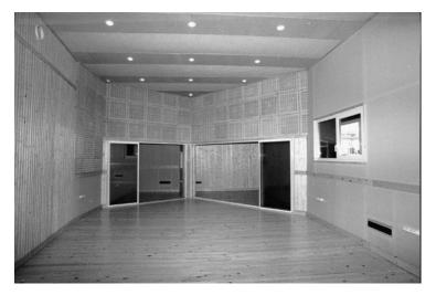
Figure 7.1 Dobrolyot Studio, St Petersberg, Russia (1996). Note the ex-Soviet era perforated diffusers over the glass doors and on the adjacent left-hand wall. (See also on the front cover.)
