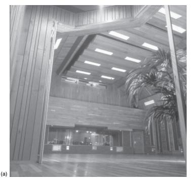
**Figure 7.8** (a, b) (a) The large, variable acoustics room at Olympic Studios, London, UK, designed by Sam Toyashima. The ceiling panels can be raised and lowered electrically, from the control room, enabling the acoustic changes to be monitored as they occur
