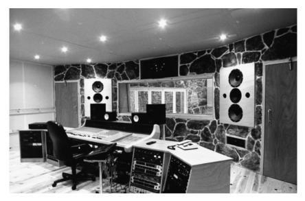
**Figure 13.10** The control room at Area Master Studios, Vigo, Spain, designed by the author, showing the vertical alignment of the drivers in the Reflexion Arts loudspeakers (1997)
