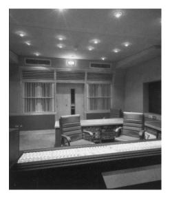
Figure 17.2 Rear end of a 'Live End-Dead End' room showing the diffusers. BBC, Maida Vale
