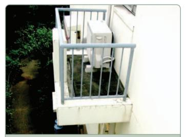
Overridden design intent Every apartment in this same Japanese eco development has installed air-conditioning on the balcony (which was intended to be for airing clothes, as an energy efficiency and health measure) (Photo: the author)
