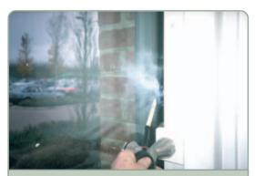
Simple leakage test using a smoke pencil Smoke escapes through inadequately sealed windows (Photo: Bill Bordass)
