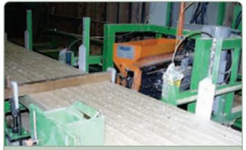
Sohm Diagonaldubelholz Factory, Austria Factory construction of solid timber panel, 8–30 cm thick, up to 16 m long and 620 cm wide. Glueless bonding using dowels rammed under pressure into holes drilled orthogonally in two directions to resist movement. Wall elements have one side of finished quality, making a high quality, ecologically sound and healthy building material (Photo: the author)
