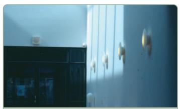
**Control** These lights are on despite the incorporation of daylighting. Energy savings from daylighting come from appropriate behaviour as well as design! (Photo: the author)
