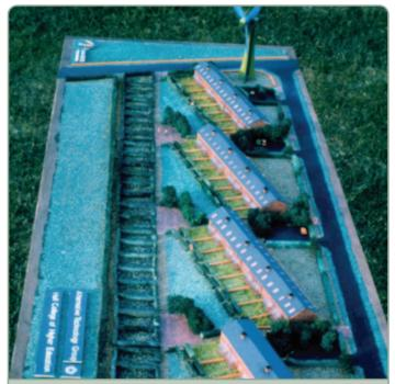
Hull Terraces Project led by Howard Liddell at Hull School of Architecture in the 1970s to optimise building orientation (Photo: Howard Liddell)
