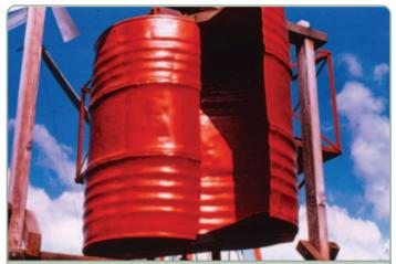
Savonius Rotor 1970s (Photo permission: Centre for Alternative Technology)
